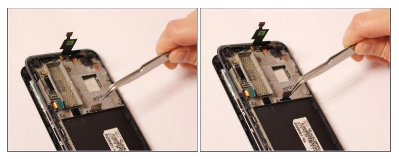
When you are putting the front and back portions of the phone back together, make sure you don't forget to pull the LCD ribbon cable through the corresponding slot to connect back to the motherboard.
