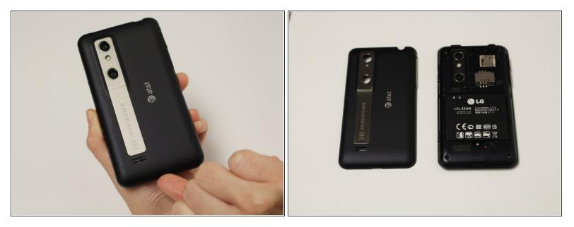
• Pry the back cover off of the phone with your fingernail. There is a notch located at the bottom of the phone for improved leverage.
