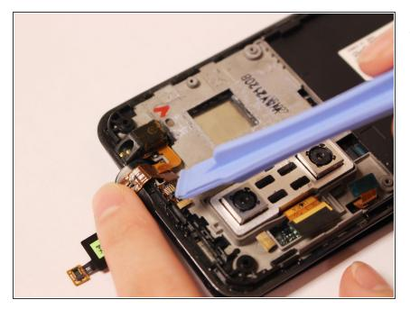
Using the plastic opening tool disconnect the ribbon cable connected to the headphone jack assembly.
