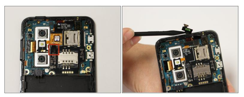
Using a spudger or plastic opening tool, gently disconnect the ribbon cable attached to the black SIM card board.
