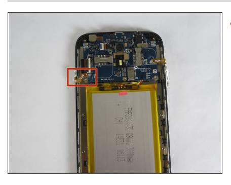
The power button is located on the rear-left side of your phone just above the battery.
