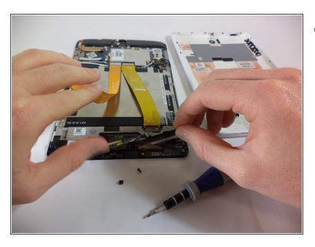
Remove the IO board carefully.
