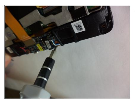
Remove the two Phillips PM1.5×4.0 screws that secure the I/O board to the display panel assembly.
