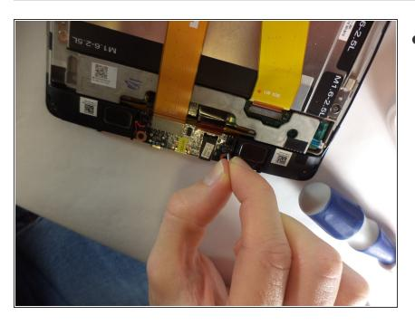
Disconnect the speaker cables from the I/O board
