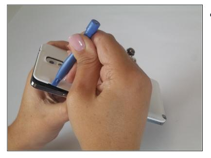
Insert a fingernail or plastic opening tool in the gap between the rear case and the base of the phone.
