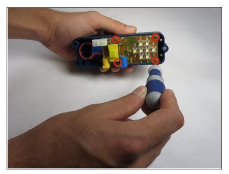
Unscrew the Phillips four #0 15mm screws to free the motherboard from the casing.
