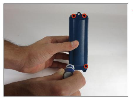
To open up the casing, you will need to unscrew the four Phillips #0
