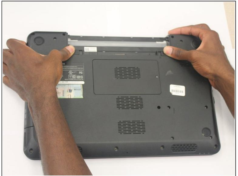
**⚠** Make sure laptop is powered off before removing the battery.
