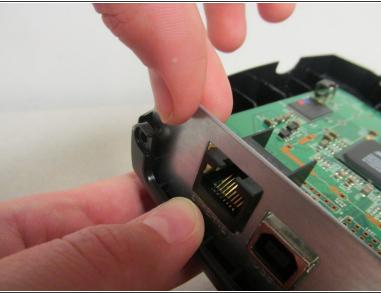
After opening the router, grab the upper left corner of the sliver face plate and gently pull the motherboard out of the slot from within the case.
