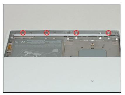
Remove the four 3 mm indicated Phillips #00 screws from the front wall of the battery compartment. When working from the left, remove the 2nd, 4th, 7th and 9th screw.
