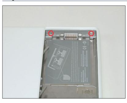
• Remove the two 6 mm Phillips #00 screws from either side of the right wall of the battery compartment (not the ones closest to the battery connector).
