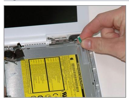
• Lift the Bluetooth antenna board from the right side of the optical drive.
