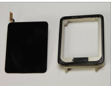
After using the pick to loosen the adhesive, simply pull the display assembly up from the metal bezel.
