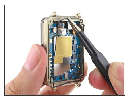
Use a pair of tweezers to remove the gasket that lies embedded in a groove that runs around the perimeter of the front half.
