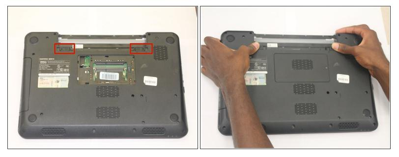
Make sure laptop is powered off before removing the battery.
