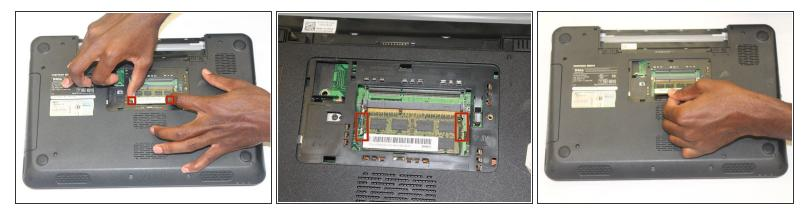
• Snap open the bottom memory clips and remove the memory drive they hold in.
