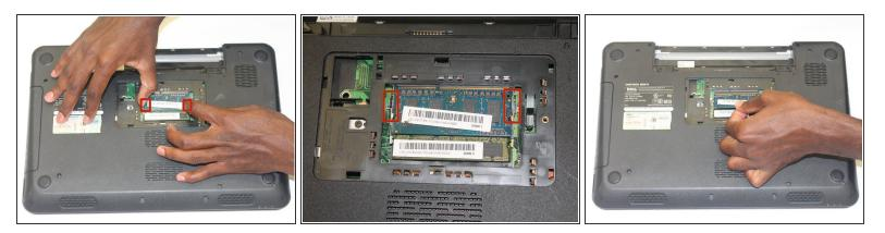
• Snap open the top memory clips and remove the memory drive they hold in.
