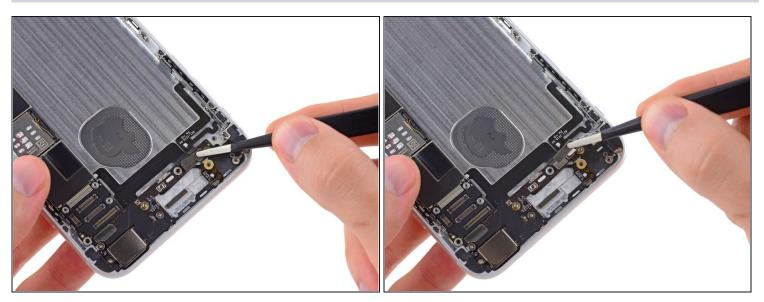
• Use a pair of tweezers to peel the single adhesive tab that resides on top of both the power button and audio control/rocker switch cable connectors.
