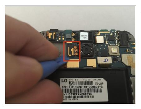
Using a plastic opening tool, pry the connection between the cable and the phone. With even pressure the cable should disconnect from the logic board easily.
