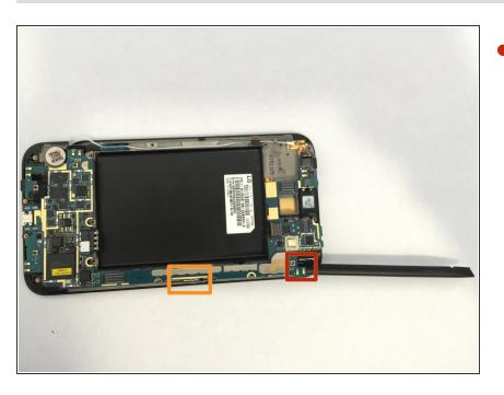
The logic board is connected to the under side of the phone with a bit of adhesive. Using a spudger, place it under the logic board from the top right corner and gently slide it toward the center orange mark where the adhesive is. Apply a little bit of pressure parallel to the logic board and the Logic board should loosen from the phone.
