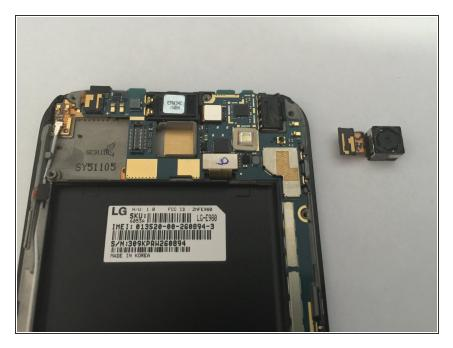
After removing the the Ribbon Cable, the Rear-Facing Camera should be able to be removed easily with your fingers.
