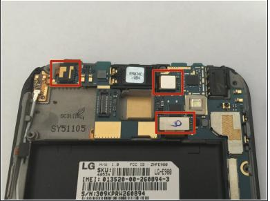
Use the plastic opening tool to disconnect the 4 ribbon cable connections and the antenna attached to the logic board.
