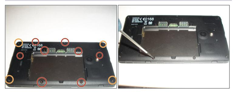
• To access the inner components of the device, remove the various screws. Keep them separate, and organize them by size.
