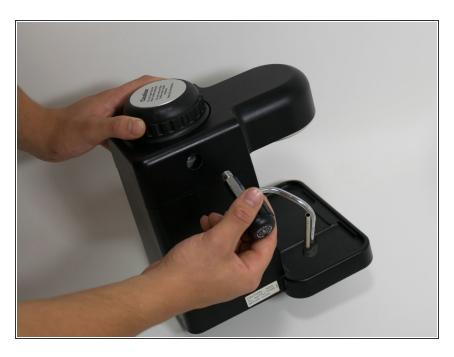
• Remove the steamer attachment from the machine.
