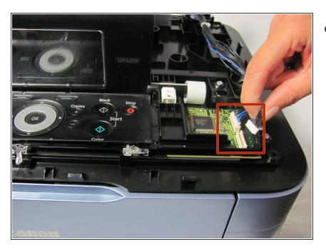
Unplug the two wires shown at the right of the command screen
