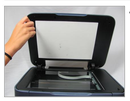
Open top lid of the printer to reveal the scanner
