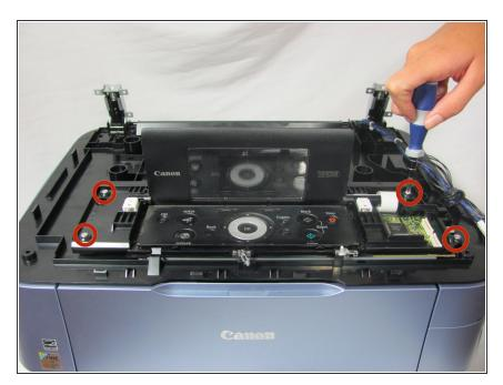
Unscrew the four screws shown to detach the command screen from the printer
