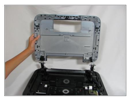
After these two panels are separated, set the top panel to the side for now
