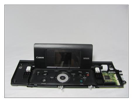
Take the detached command screen off of the printer and replace.
