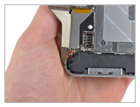
Remove the 1.9 mm Phillips screw securing the bottom of the logic board to the inner case.
