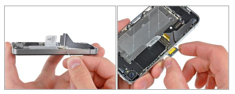
Use a SIM card eject tool or a paperclip to eject the SIM card and its holder.
