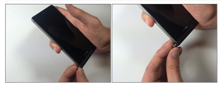
Pull and twist the pin near the bottom left-side of the phone to remove it from the headphone jack.
