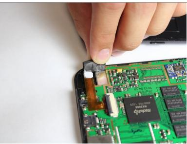
Remove the black pad on the back of the camera by peeling it off.
