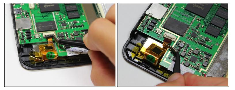
Use the tweezers to lift the grey connector, located near the reset button, up from the beige housing. It should rotate up, and allow you to slide the ribbon out from under the connector.
