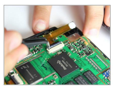
Use the tweezers to lift the grey connector, connecting the camera ribbon to the circuit board, up from the beige housing. It should rotate up, and allow you to slide the ribbon out from under the connector.
