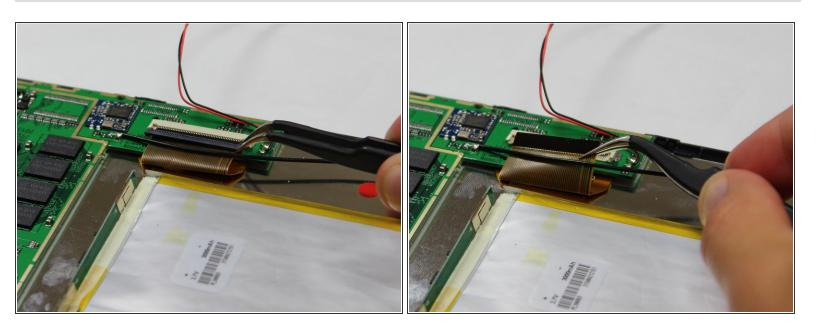
• Use the tweezers to lift the grey connector, located near the battery and speaker, up from the beige housing. It should rotate up, and allow you to slide the ribbon out from under the connector.
