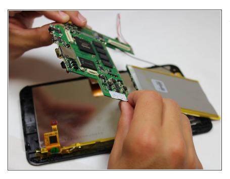
Lift the circuit board and the battery off of the front panel.
