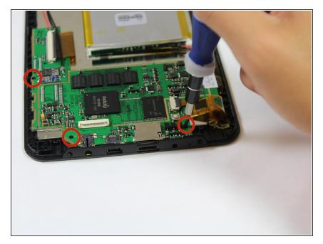
Remove the three 4.0mm screws holding down the circuit board with the Phillips #00 screwdriver.
