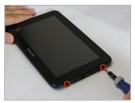
Unscrew the two 4.0mm Phillips head screws found near the ports at the bottom of the device using a PH #00 screwdriver.
