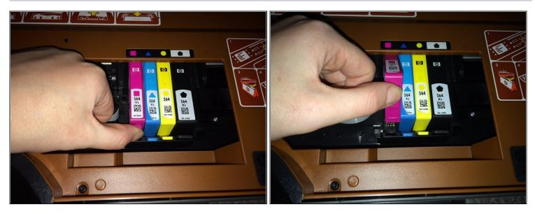
• Press down gently on the front tab of the ink cartridge that needs replacing and then lift up.
