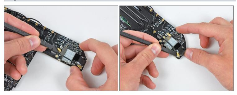
• Use the flat end of a spudger to pry the antenna connectors up off the AirPort/Bluetooth board.
