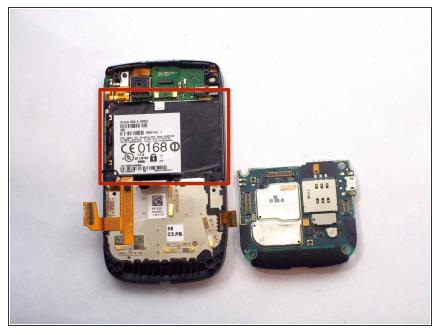
Remove the black sticker located above the logic board that contains the phone's serial number
