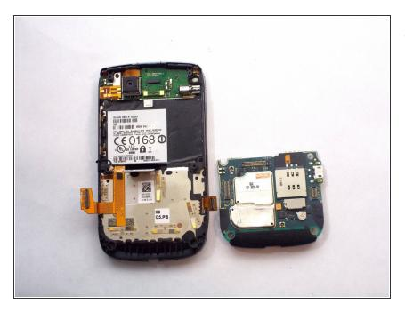
• The logic board will easily pull straight out.
