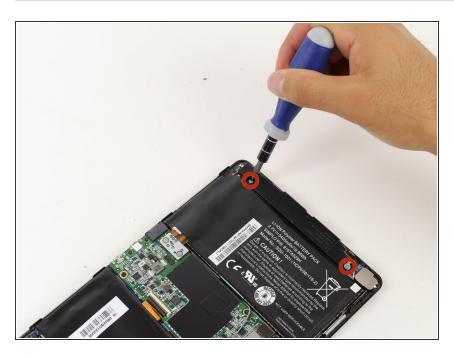
Remove both 1.5x4.25mm Phillips screws from the right speaker bar by using the Phillips Screwdriver.
