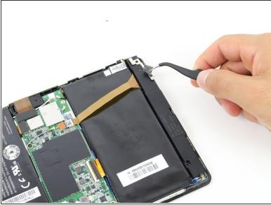
Peel off the stickers holding the left speaker in place with a tweezer or by using your fingers
