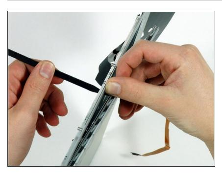
Place the upper casing on its edge and use a spudger to push the keyboard away from the casing, poking the spudger through the central keyboard screw hole. Grasp the keyboard as it separates from the casing.
