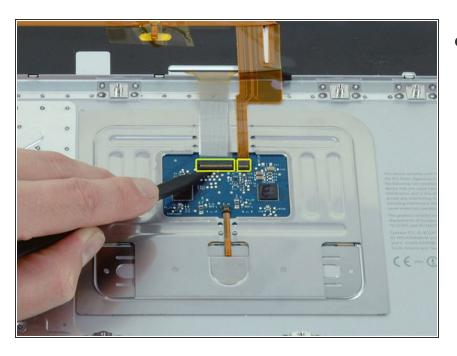
Use the tip of a spudger to flip up the black plastic flaps locking down the keyboard and keyboard backlight ribbon cables.
