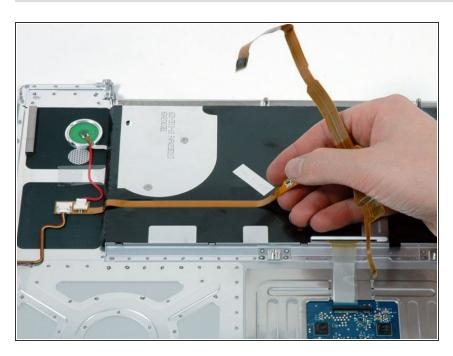
Carefully peel up the orange ribbon cable which carries the power and sleep signals.
