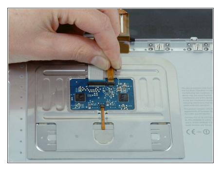
Slide the orange keyboard backlight ribbon out of its connector.
