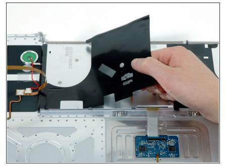
Peel up the two black protective sheaths on the bottom of the keyboard. It is not necessary to fully remove these, but only to peel them back enough to access the screws beneath.
