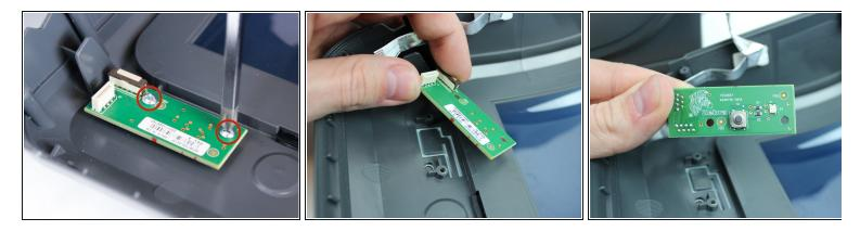
• Remove 2 7.51mm Phillips screws holding the circuit board onto the device casing.
