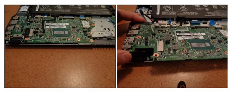
• Taking care not to catch the motherboard peripherals such as the USB, microphone jack, and DCin on the left hand side of the motherboard on the chassis pull out the motherboard by moving it a little to the right and then pulling up.
