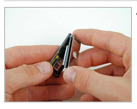
Lift the bottom of the rear case and remove it from the rest of the iPod.
