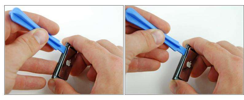
Insert an iPod opening tool into the newly widened gap, and pry the rear case up and away from the front case.
