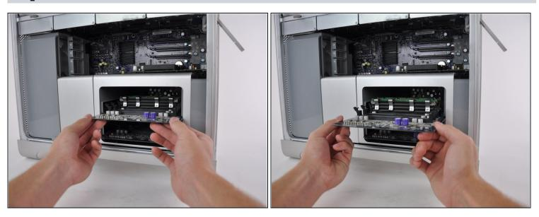
• Pull the RAM tray out of the case by using both hands holding the edge of the ram board as shown.
