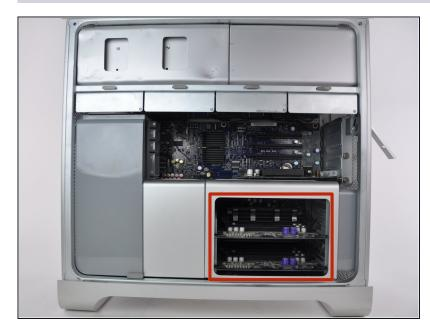
• Locate the two RAM trays at the bottom of the Mac Pro.
