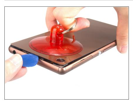
Insert guitar pick into the gap and slide to cut the sticker around the back cover.
