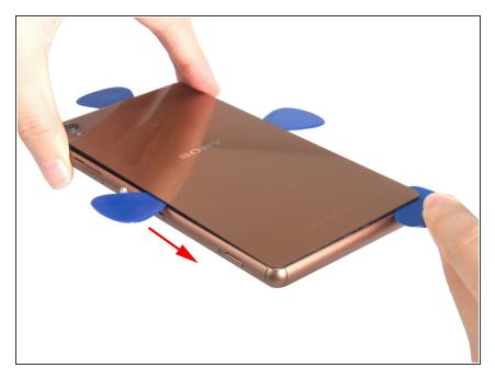
Especially the left side, you'd better handle as the direction we marked or you are likely to break the flex cable on the left bottom corner.
