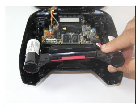
Pull the battery apparatus out once all cables are removed.
