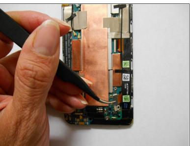
Disconnect the battery by prying the metal cover straight up.
