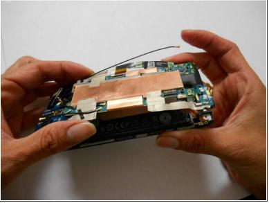
Lift the motherboard, but don't try to remove it completely yet.
