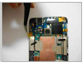
Use tweezers to remove the yellow tape covering the flex cable connectors (total of five).
