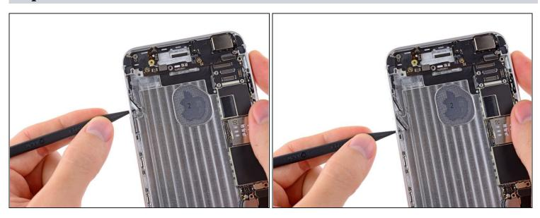
• Use the tip of a spudger to push the audio control and rocker switch buttons out of their recess on the rear case.
