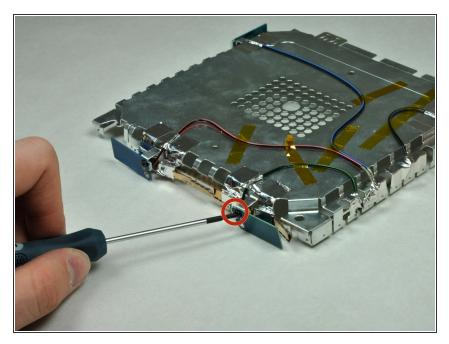
Remove the 5 mm Phillips #00 screw holding the blue antenna to the logic board.
