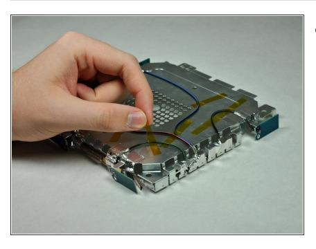
Remove the tape that attaches the wire to the logic board.
