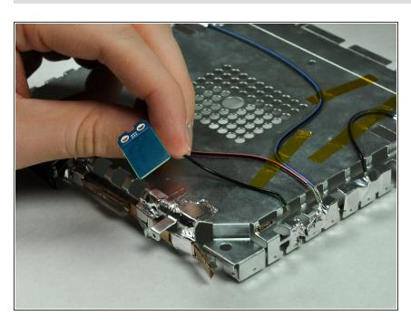
Finish by lifting the antenna out of its position. The antenna and wire should be free from the logic board at this time and ready for replacement.
