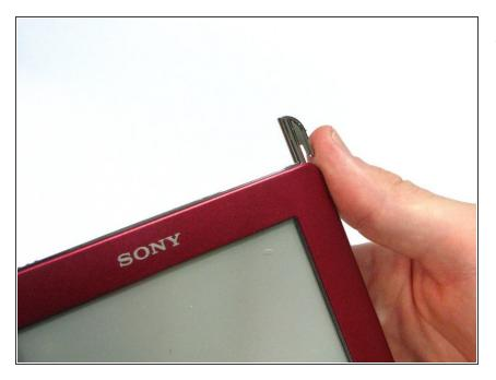
Remove the stylus from the device.
