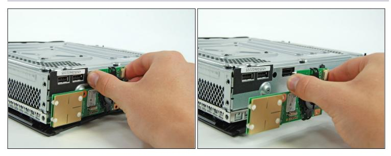
(*i*) The RF module is still connected to the Xbox by a large USB-type connector.
