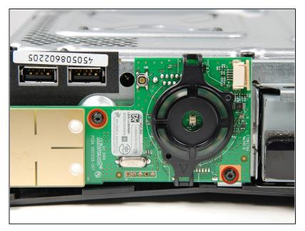
• Remove the two 5.6 mm T8 Torx screws securing the RF module to the metal case.
