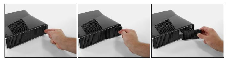
i Orient the Xbox 360 S so that the bottom of the console is facing toward you.
