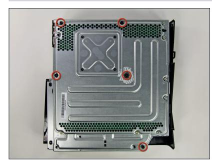
• Remove the five 55.5 mm T10 Torx screws securing the right case to the metal frame.
