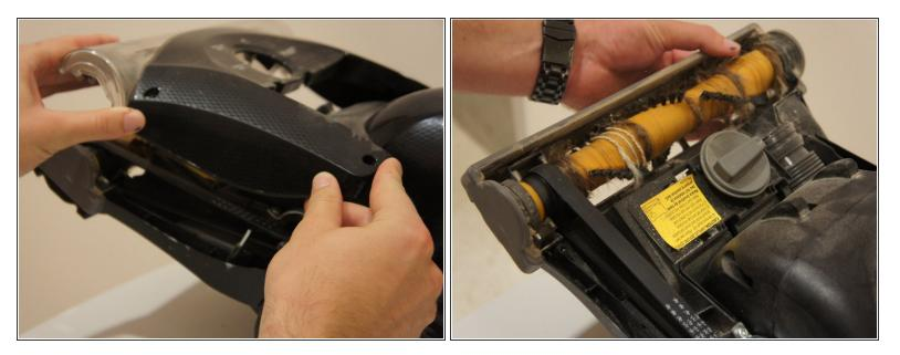
• Remove the brush cover from the vacuum base, by pulling straight up.
