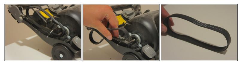
• Remove the belt from around the motor.
