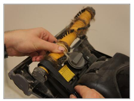
• Once the brush roll is displaced from the base, detach the belt from the brush roll in order to clean the brush roll.
