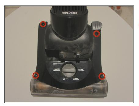
Using a Phillips #2 screwdriver, remove the four screws from each corner of the brush roll cover.
