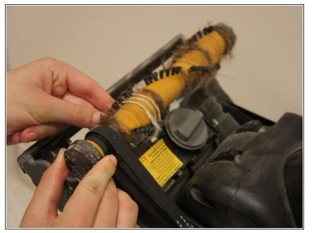
After one end is displaced, remove the other side by pressing firmly upwards from below the the brush roll.
