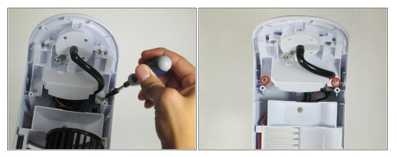
Remove the two 3mm screws found just below the top of the device using the Phillips #0 Screwdriver.
