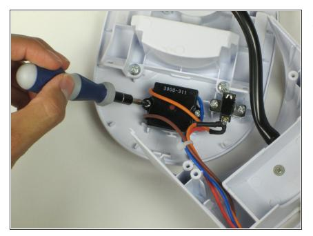
Remove the two 3mm Phillips #0 screws from the back of the black dial box.
