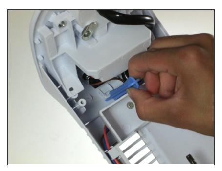
Pry off the control panel by forcefully lifting the tab located inside the front of the fan with the plastic opening tool.
