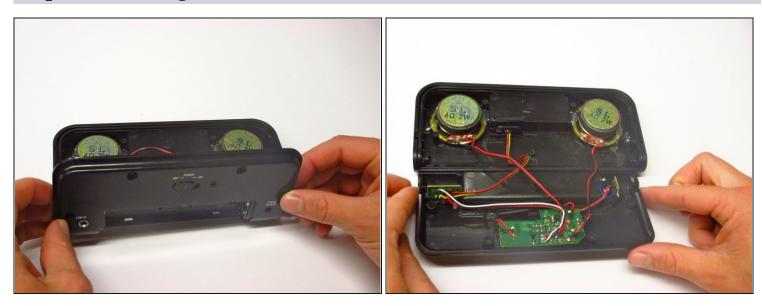
• Remove the back cover carefully; there are many wires that connect it to the device.
