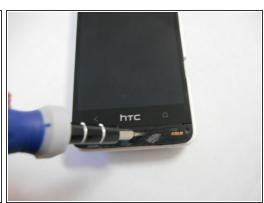
Remove the screw under the speaker cover using a T6 Torx screwdriver.
