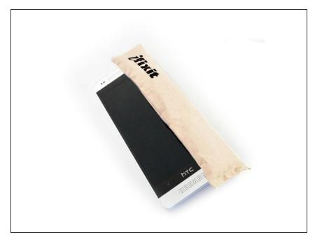
Use an iOpener or hair dryer to apply heat to the lower speaker grille, in order to soften the adhesive underneath.
