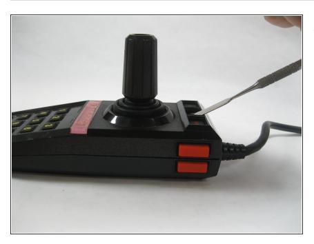
Using a plastic or metal spudger, pry open the face of the button module.
