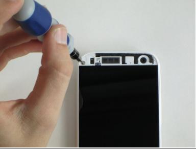
Remove the 2mm screw with a T5 torx screwdriver head from the iFixit tool kit.
