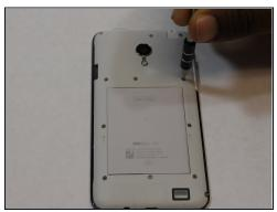
Using one of the small Phillips screwdriver bits provided unscrew the 11 screws present on the protective plastic plate under the device case.
