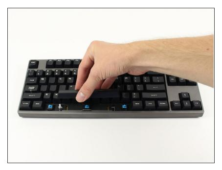
Pull the large keycap upward with your fingers until the cap separates from the plastic rings underneath the cap. If the metal bar beneath the cap comes loose during removal, snap it back in place.
