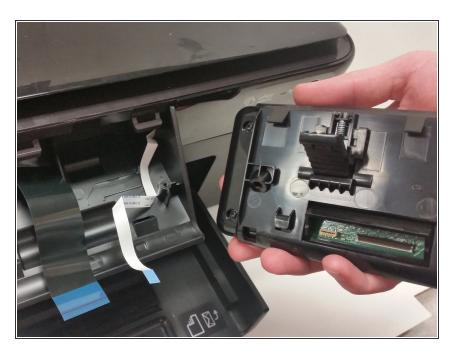
Once the ribbon cables have been removed, your screen should be free of the printer.
