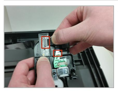
Remove the two ribbon cables from the scanning light.
