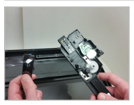
The scanning light is now removed from the printer.
