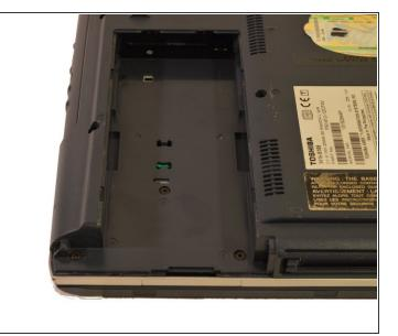
Lift the battery straight up, out of the computer.
