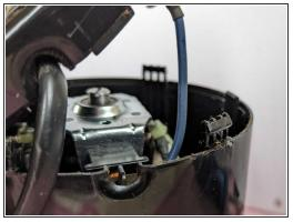
Wedge the spudger between the flat side of the E-clip and the outside wall of the slot. Then, loosen
