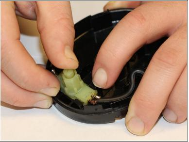
The trigger button is held in with light tension clips. Gently pry them back to release.
