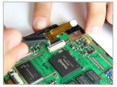
• Use the tweezers to lift the grey connector, connecting the camera ribbon to the circuit board, up from the beige housing. It should rotate up, and allow you to slide the ribbon out from under the connector.
