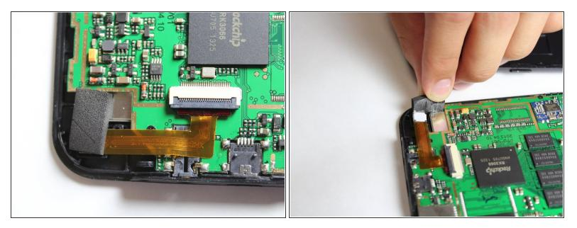
Remove the black pad on the back of the camera by peeling it off.
