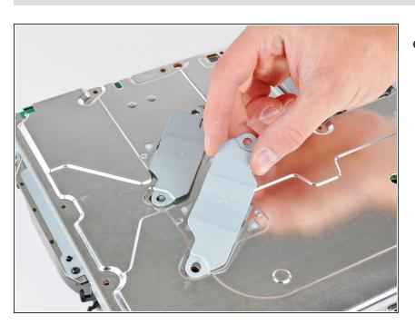
Remove the two heat sink clamps from the bottom of the motherboard assembly.
