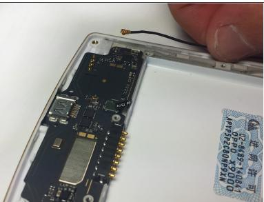
With your fingers, gently pull upwards on the WiFi antenna near the connection on the smaller motherboard until the antenna is no longer connected to the bottom motherboard.
