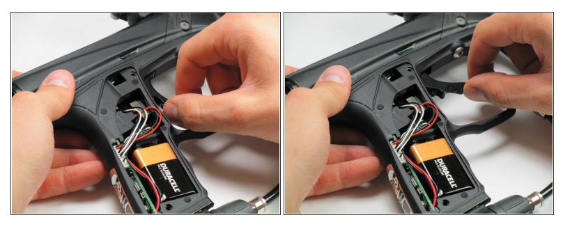
Pull out the trigger by grabbing the bottom and slowly rotating outwards.
