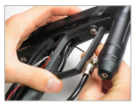
Use a hex key to unscrew the middle screw on the top of the trigger.
