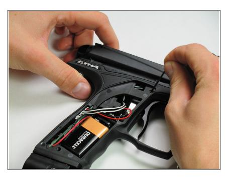
Use same hex key to push through trigger retention pin on the side of the gun.
