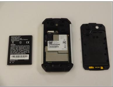
Place index finger at the top edge of the battery and gently lift upwards. The battery will slide cleanly out of the phone. The SIM card slot lies under the battery.
