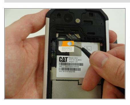
The old SIM card is removed and replaced with the new one. The phone can be reassembled by following these steps in reverse order. To reassemble your device, follow these instructions in reverse order.
